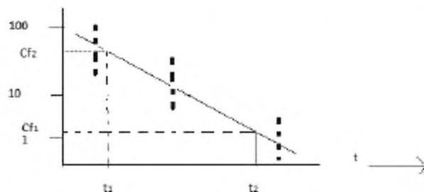
$$k_2 = \frac{\ln(C_{f1}/C_{f2})}{t_2 - t_1}$$
